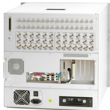
Dewetron 908 Ground Station Computer with integrated BNC Rear Panel
