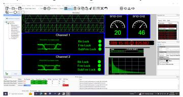
a Chapter 7 RF or PCM Simulator to generate outgoing telemetry data from stored Chapter 10 files.
