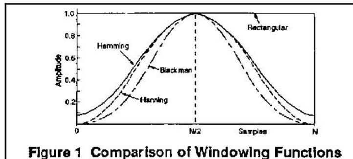
**Figure 1 Comparison of Windowing Functions**
