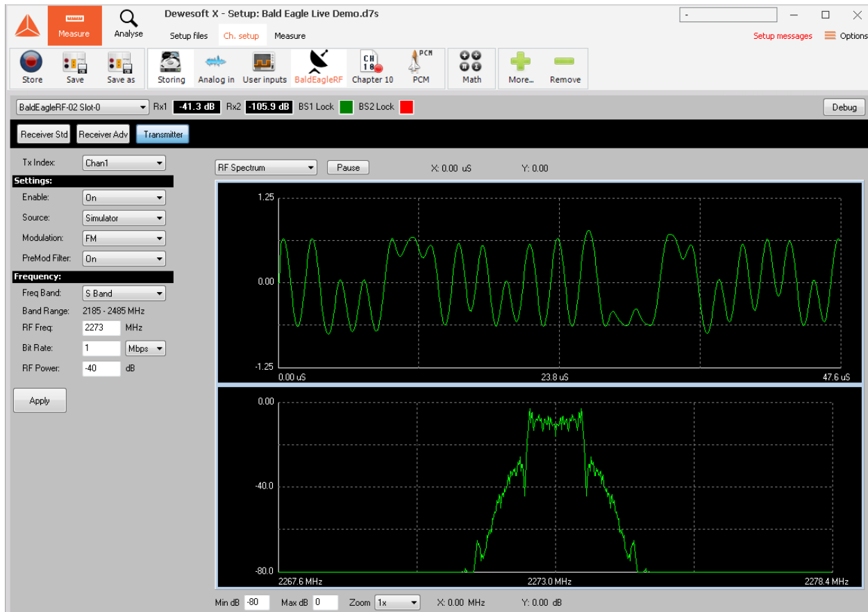
Figure 12 BaldEagleRF Plug-In Transmitter Channel Setup
