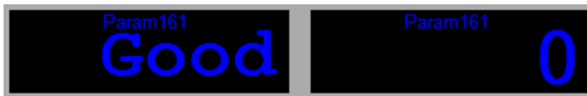
Figure 122 – Lookup Display and a Meter Display
